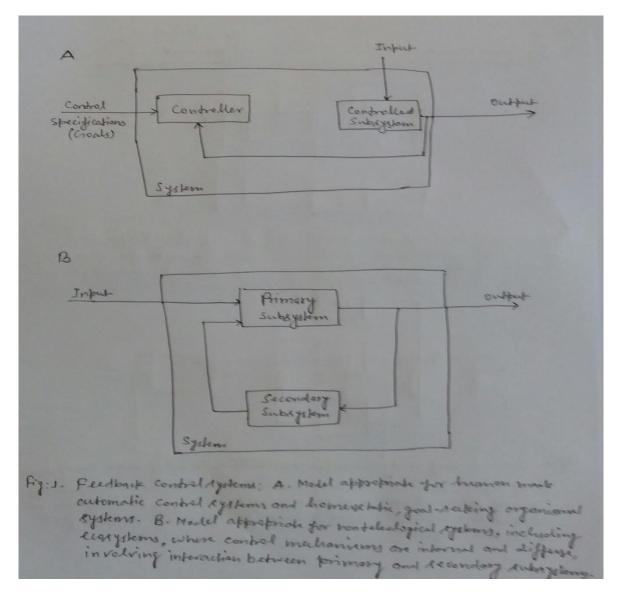
Principles of cybernetics are modeled in figure 1, which compares a goal-seeking automatic control system with specified external control as in a mechanical device (A) with a non-teleologic system with diffuse subsystem regulation as in ecosystem (B). In any case, control depends on feedback, which
