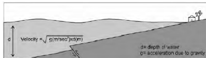
Figure 2. Cartoon diagram illustrating the mathematical relationship between depth-velocity relationship of Tsunami wave.
